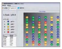
Each kernel is color coded for the five-level ranking scale.
